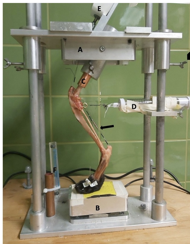
Figure 1. Limb press. A = top plate; B = pedestal; C = copper tube holding the femoral shaft; D = spring mechanism to avoid slack; E = force gauge; and F = radiographic magnification marker (Biomedtrix, Whippany, NJ, USA). Arrowhead = screws to fixate the top plate. Arrow = Achilles tendon mechanism.
